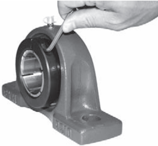
Fig 14.11 Installation of NU-LOC units
